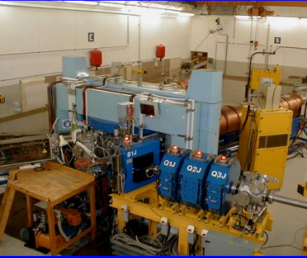
K8 Injector cyclotron 1
